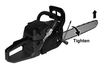
While lifting the chain guide, turn the content screw to apply correct tension to the chain. Then lock the crankcase nuts.
