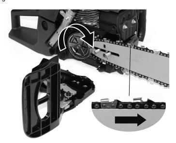
5) Reinstall the cover and screw it the two screws provided.
